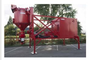
Reducing noise pollution and protecting the environment were important considerations when designing the Vacu-Press®. The double filter system has such a high degree of separation that the emission value is extremely low and pollution of the pump is limited.
